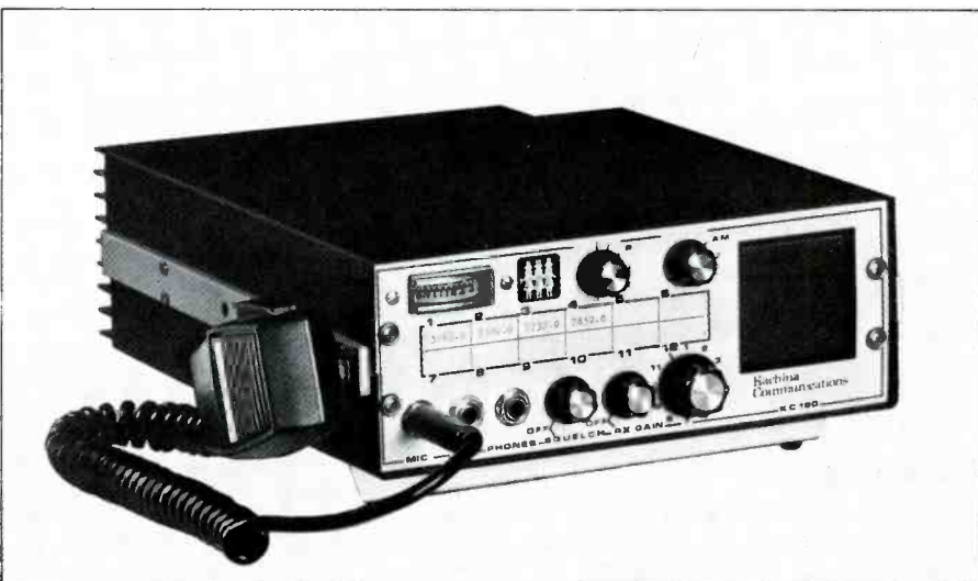
Kachina Communications, Inc. produces this 100 watt transceiver, which can operate on any frequency between 2 and 12 MHz.
