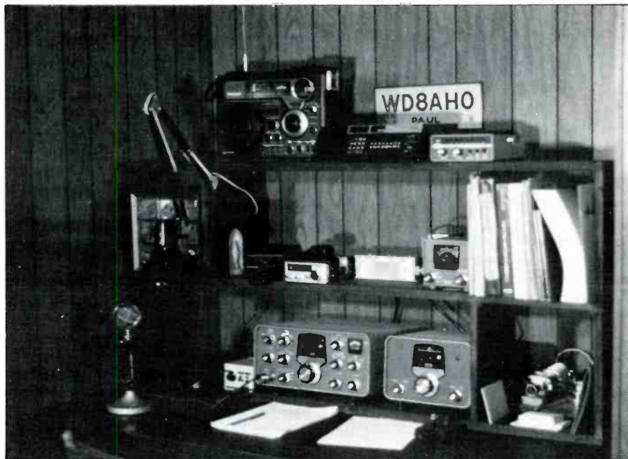
The shack of Paul DeNapoli. Equipment shown is Panasonic 2600, Regency 16 channel programmable scanner, Sonar-Scan 8 channel scanner, President Model 10 40-channel CB, Drake TR-33 two meter transceiver, and a Heathkit SB-101. All equipment can be run by the Amcon I system. (Photo courtesy ENCON Corporation)
